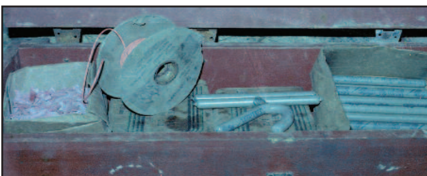
Modern TOVEX dynamite. It was waterproof and very safe until you put a blasting cap in it; then it became a very powerful tool for blasting rock.
