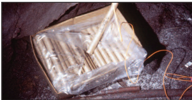
Box of stick powder. These sticks were hard, and you could break a stick in half if you needed less power in your blasting.
