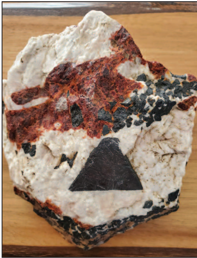
This is good chunk of zinc ore. The franklinite is black, the zincite is red, and the white mineral is calcite.
