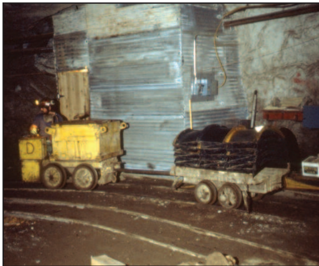
This photo shows our small "motor" or engine in use on the 1850 level, while the mine was operating. This "motor" was used for hauling small loads of equipment back and forth underground. It was too small to haul our loaded ore cars, but worked just fine for moving smaller equipment.
