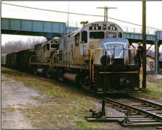
CAPTION: The last locomotives that LHR purchased were ALCO Century C420's, built in Schenectady, NY. Locomotive #29 was the last of the nine purchased in the early 1960s. In this photo, #29 idles under the mighty Franklin Viaduct, after picking up a string of ore cars from Sterling Hill, waiting to head out onto the main, and make the run to Allentown, PA.
