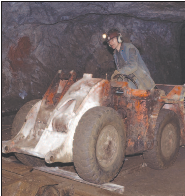
John Kolic, at a shaft station in the Sterling Mine, preparing to place a Load-Haul-Dump Loader (LHD) onto a carrier for transport to another level.
